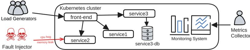
Fig. 4. Overview of our setup for microservice systems.
